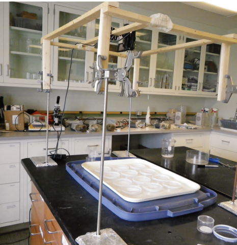
The laboratory video setup shown here is for tracking bed bug movement.
